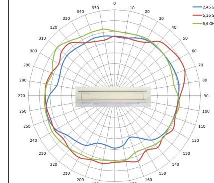
Azimuth WLAN2 (5dB/div)
