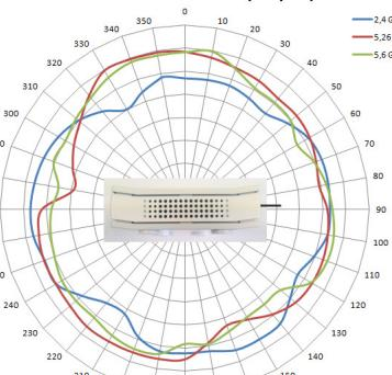
Azimut WLAN2 (5dB/div)
