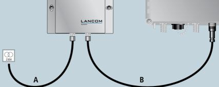
(3) Connect the output cable (B) of the LANCOM OAP-380 PSU with the voltage input connector on the LANCOM OAP-382. Leave some slack in the cable to compensate for heat-induced changes in the cable length. Arrange the cable such that the lowest point of the loop encourages water to flow away and not get into the housing.
