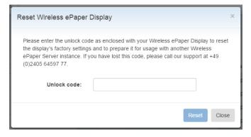
If a Display is reset after it was already associated with another Wireless ePaper Server, it must first be registered with the new server. Then it must be reset, deleted and registered again.
