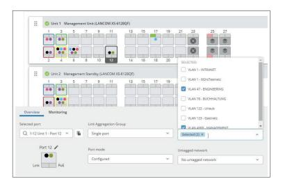
LAG setup for stackable switches
