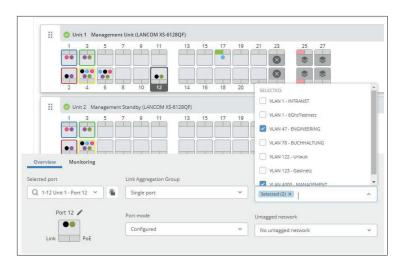
LAG setup for stackable switches
