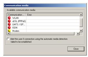
The available communication media are displayed with yellow signal lamps and the automatically selected with a green signal lamp.
